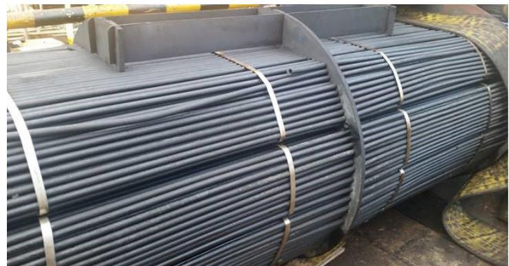
Preheater train heat exchanger E-2505F decontaminated (0% LEL, 0% H<sub>2</sub>S, 0% benzene) using Vapor-Phase method in 7 hours after a viscosity wash with LCO and Rezyd-HP Z71 was circulated for 16 hours.\*
