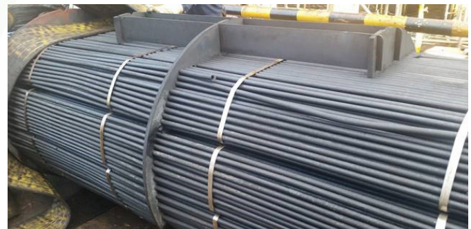
● Preheater train heat exchanger E-2505F decontaminated (0% LEL, 0% H 2 S, 0% benzene) using Vapour-Phase method in 7 hours after a viscosity wash with LCO and Rezyd-HP Z71 was circulated for 16 hours.**
