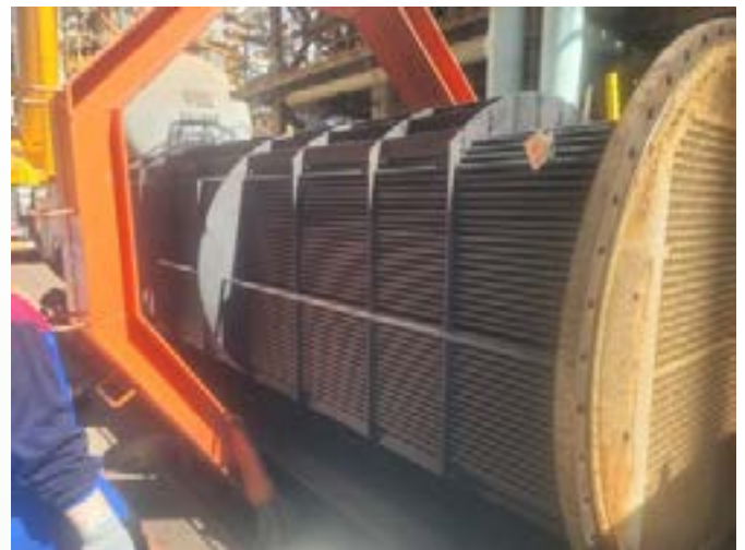
● PULLED SLURRY HEAT EXCHANGER AFTER REZYD-HP® TREATMENT
